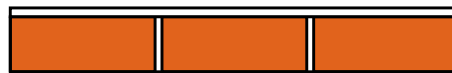
Figure 55 NCC Deemed-to-Satisfy Wall Systems for NT: Rendered single leaf brickwork, 80mm clay bricks
