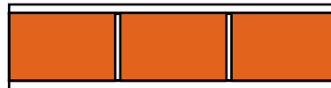
Figure 49 NCC Deemed-to-Satisfy Wall Systems (ACT, NSW, QLD, SA, TAS, VIC, WA): Rendered single leaf brickwork, 150mm clay bricks
