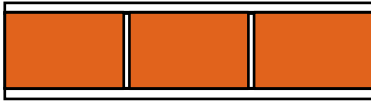
Figure 50 NCC Deemed-to-Satisfy Wall Systems (ACT, NSW, QLD, SA, TAS, VIC, WA): Rendered single leaf brickwork, 220mm clay bricks
