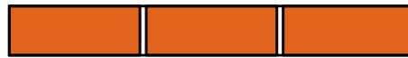
Figure 54 NCC Deemed-to-Satisfy Wall Systems for NT: Single leaf brickwork, 110mm clay bricks
