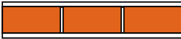
Figure 51 NCC Deemed-to-Satisfy Wall Systems (ACT, NSW, QLD, SA, TAS, VIC, WA): Rendered single leaf brickwork, 110mm clay bricks
